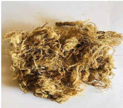
Plate III: Banana stem fibres extract after treatment
