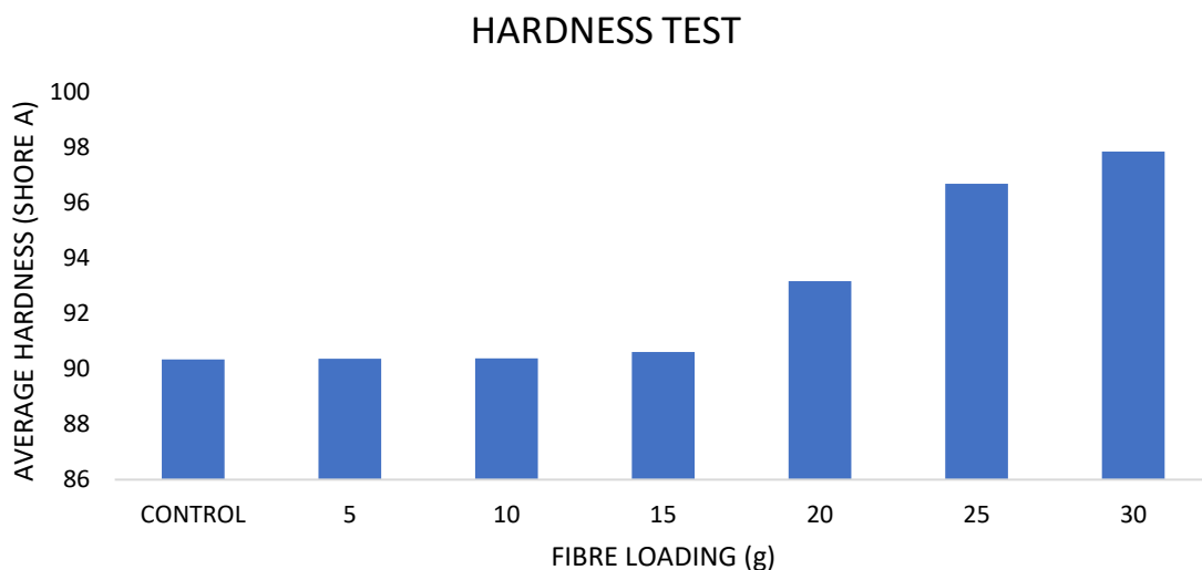
Figure 1: Effect of hardness on fibre loading
