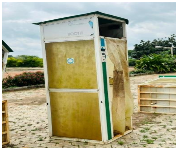
Figure 3: Image of the locally fabricated disinfectant booth by FPI
